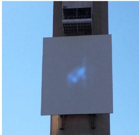
Specular reflection – 39% filter. Distance 157m on 12 x 12 m target
